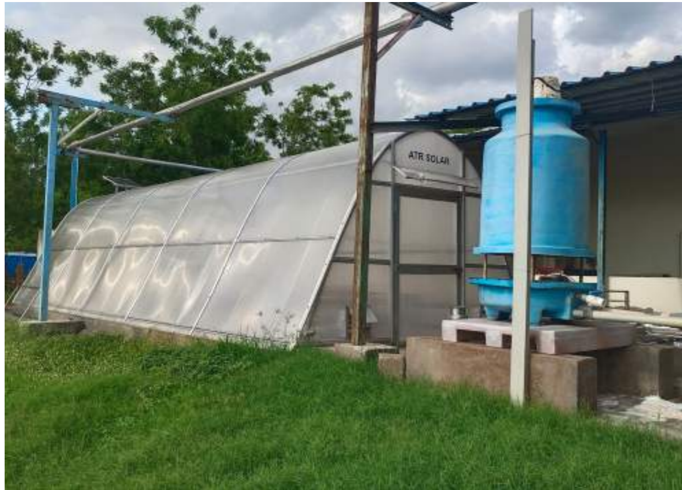
Solar dryer to upkeep the containers used in the powder processing unit in the Oonaiyur facility
